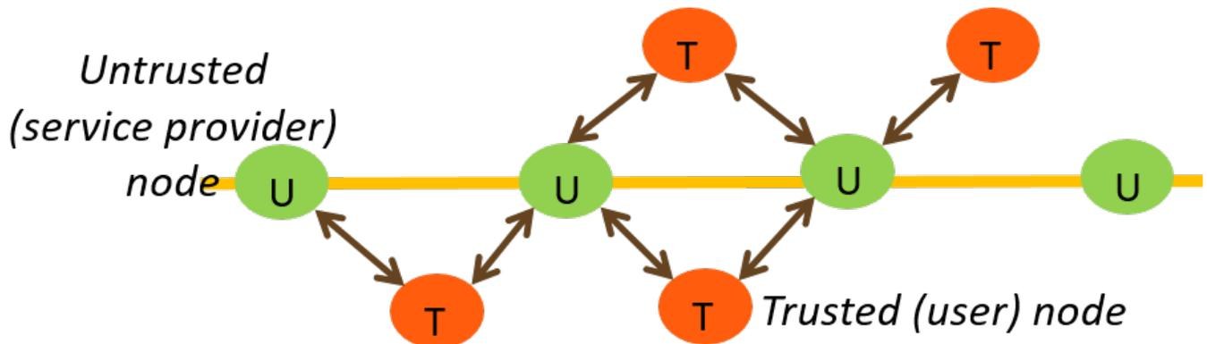
FIG. 2. The schematic of a partially trusted QKD network. We exchange a key, using, e.g., MDI techniques, between two adjacent trusted (T) nodes via the untrusted (U) node that connects them together. The key exchange between the two trusted nodes not directly linked via an untrusted node can then be done similar to that of Fig. 1.
