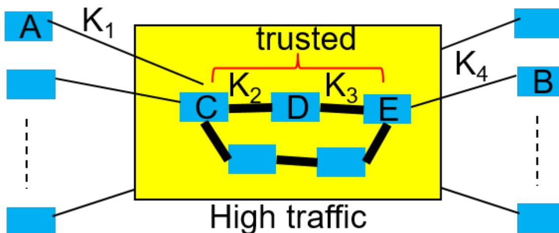
FIG. 1. The schematic of a trusted node QKD network. In order for users A and B to exchange a secret key, we need to create a secret key between any two adjacent nodes that connect A to B (e.g., C, D, and E). We can then use these keys to securely relay a key from A to B. If there are multiple paths between A and B, we can generate separate keys using each path and then combine them in the end.
